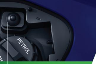
MICRO SWITCH TO KEEP THE CAR SWITCHED OFF AT TIME OF REFUELING
